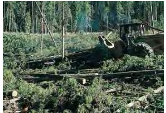
Logs are dragged by a skidder from the forest to a log landing. Rubber tired skidders or crawler tractors remain on the skid trail and winch line and chokers pull the logs to the machine. Limbing and bucking are done with chainsaws.
