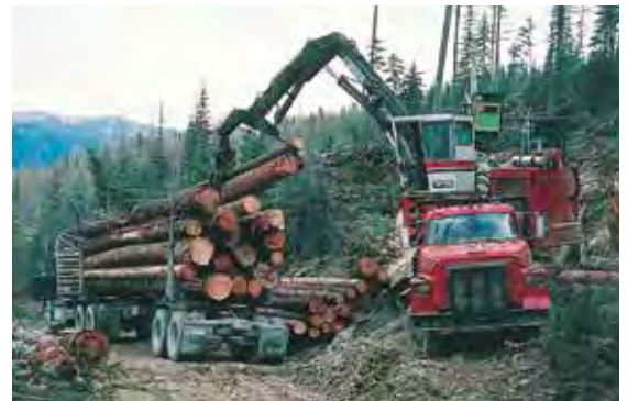
Once at the landing, a log loader moves logs onto trucks for delivery to the mill.
