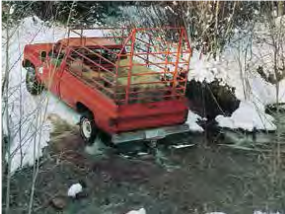
Fords are the least desirable stream crossing because of the continued disturbance to the streambed. However if used infrequently, at low flows, it may be the least impact option.
