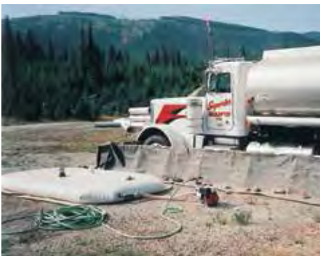
In Helicopter service areas , operators are required to provide fuel truck containment in case of accidental spills. Portable water tanks and pumps are ready for fire emergencies.
