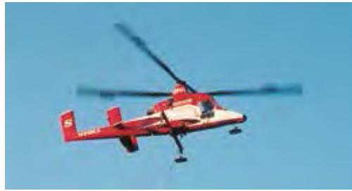
This KMAX Heavy Lift helicopter has a payload capacity of 6,000 pounds. Flight distances are typically kept to less than a mile. Longer distances are more costly. Optimum payload of each load makes the operation economic.
